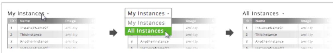
Figure 4.3 Some tables use Table Dropdowns to allow the user to determine the data to be displayed in the table
